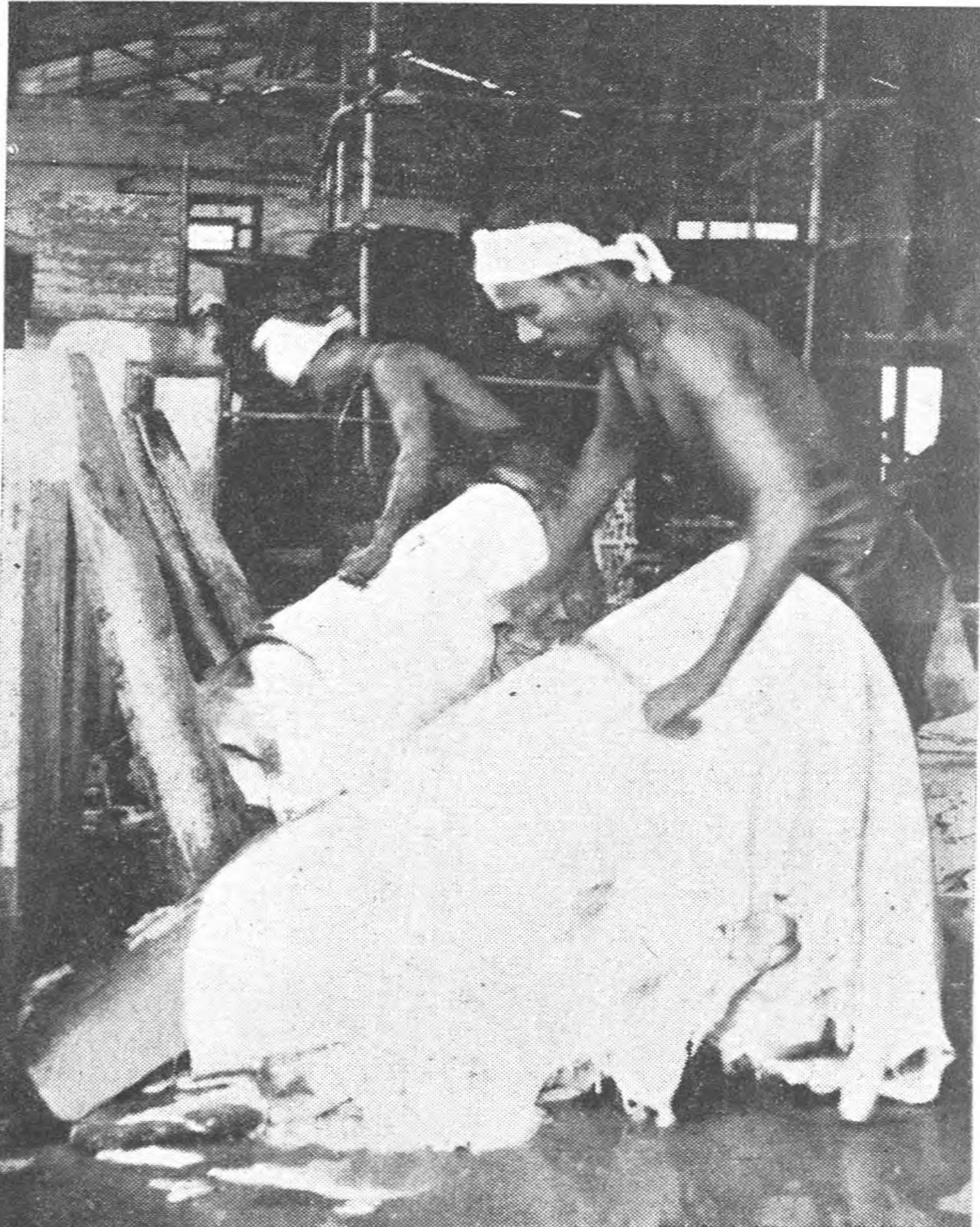
Figure 8.—Operators at Government tanning factory using scudding knives on leather
